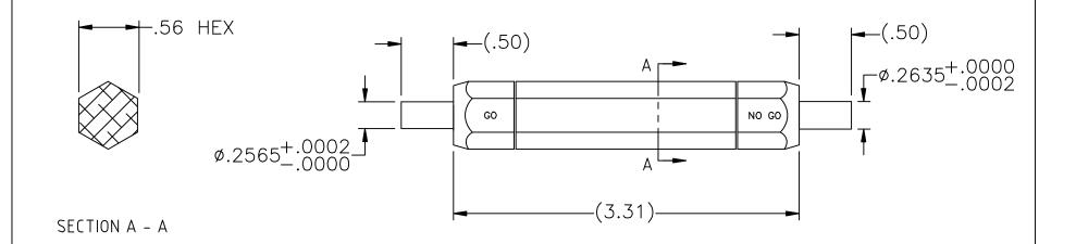
2. THIS IS A FLAT GAGE FOR HEX DIES: .125" ACROSS FLATS., BOTH SIDES NOTES: I. THIS IS AN AUTOCAD DRAWING DO NOT CHANGE MANUALLY.
